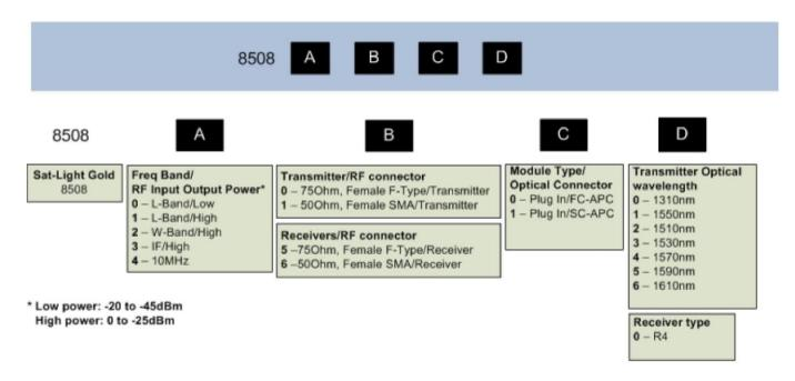
Example: Plug in module, L-band, low RF input, 1310nm laser, F-Type RF connector and FC/APC optical connector
